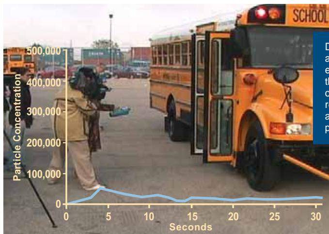
Diesel particles are virtually eliminated when the bus is run on ULSD and retrofitted with a diesel particulate filter.
