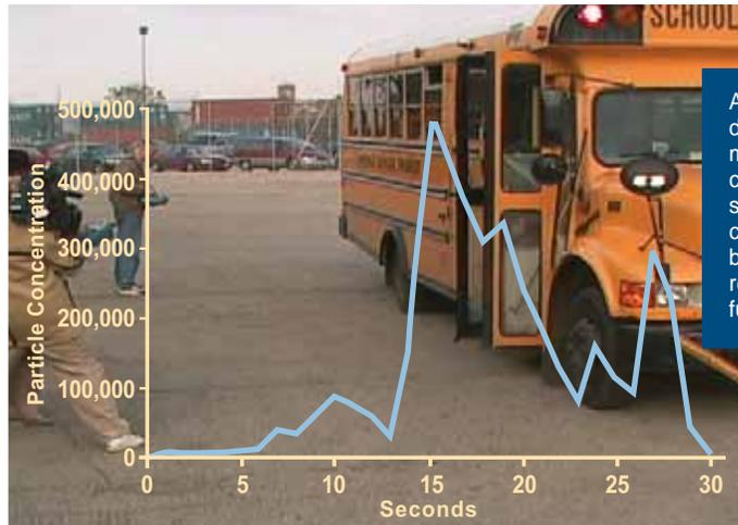
At a bus stop, diesel particles measured at the curb spike sharply from a conventional bus running on regular diesel fuel.
